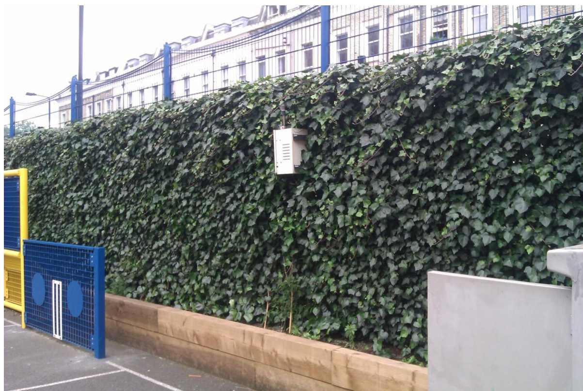
Figure 4: Osiris analyser and NO x inlet situated on the playground side of the green screen
