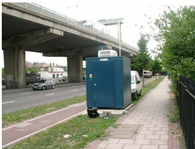
Figure 16 The Hounslow 5 roadside site that replaced Hounslow 1 during August. The site is located beside the A4 and M4 and monitors CO, NO x and PM 10 (TEOM).
