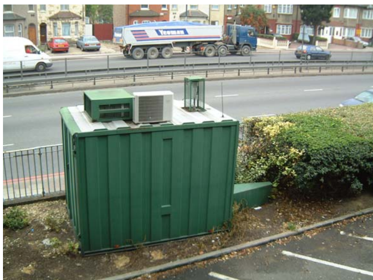
Figure 10 The Brent 4 site that joined the LAQN during June as a replacement for Brent 2. The site is located on the A406 around 300 m from the location of Brent 2. The site monitors \text{NO}_x , \text{SO}_2 and \text{PM}_{10} (TEOM).
