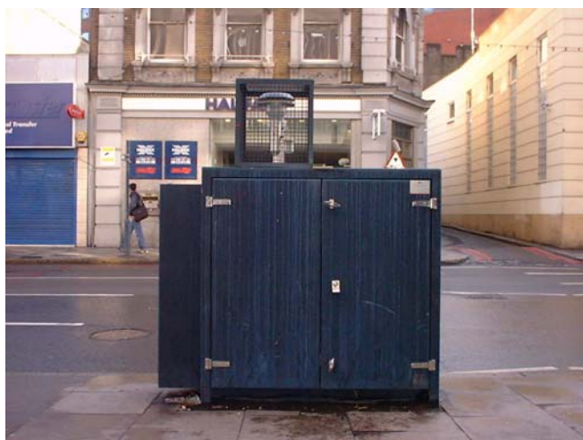
Figure 17 The Lambeth 4 roadside site that joined the LAQN in December. The site measures NO x , SO 2 and PM 10 (BAM) alongside the A23 in Brixton.
