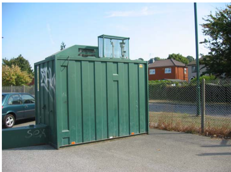
Figure 12 The Waltham Forest 3 site that joined the network during July. The site is located in a roadside location in Chingford and measures \text{NO}_x , \text{SO}_2 and \text{PM}_{10} (TEOM).
