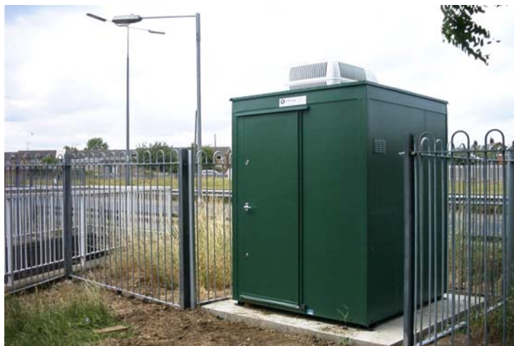
Figure 20 The Thurrock 3 roadside site joined the LAQN during August and measures NO x , SO 2 and PM 10 (TEOM).
