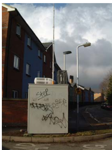
Figure 11 The Hillingdon 2 site that became fully operational during April. The site monitors \text{NO}_x and \text{PM}_{10} (TEOM) at a roadside location close to Hillingdon Hospital.
