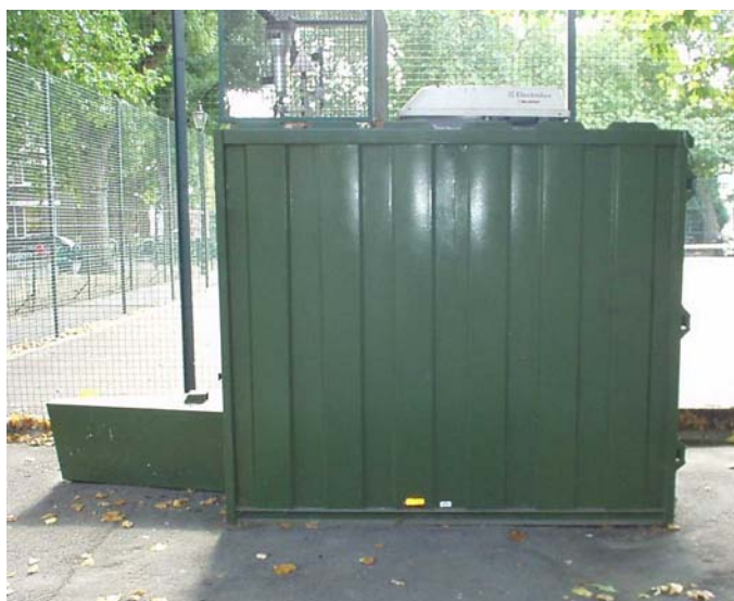
Figure 15 The Hammersmith & Fulham 2 background site that joined the LAQN during July. The site monitors \text{NO}_x and \text{PM}_{10} (TEOM).
