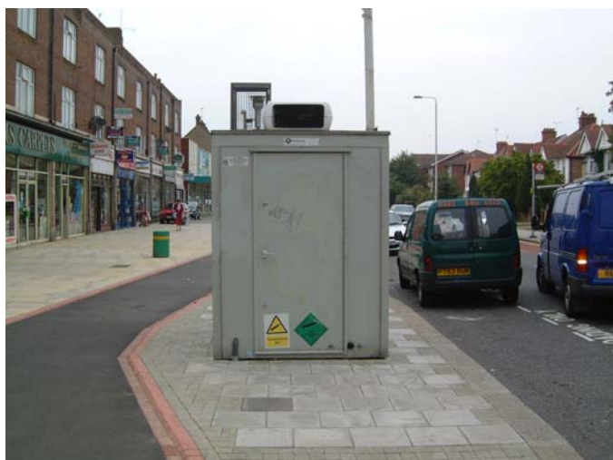
Figure 14 The Harrow 2 site that joined the LAQN during June. The site is located in a roadside location and monitors \text{NO}_x and \text{PM}_{10} (TEOM).
