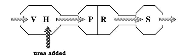
selective catalytic reduction (SCR) brings NO<sub>x</sub> down to emissions comparable with petrol engines
